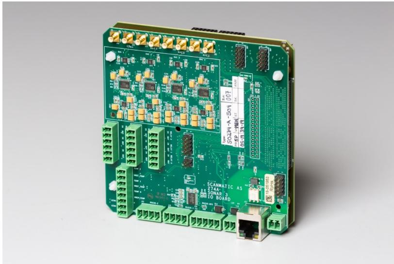
State-of-the-art electronics and robust software developed in 2018/2019 – the core of all Scanmatic hydroacoustic products
